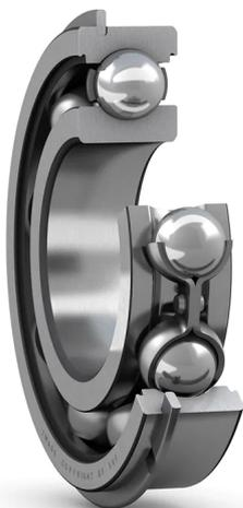
Single row deep groove ball bearings with a snap ring groove are particularly versatile, have low friction and are optimized for low noise and low vibration, which enables high rotational speeds. They accommodate radial and axial loads in both directions, are easy to mount, and require less maintenance than many other bearing types. The snap ring, fitted in an annular groove in the outer ring, facilitates axial location of the bearings within their housings.
