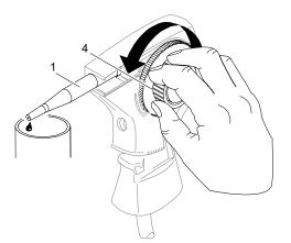
• Priming the Pump: Turn the dispensing wheel **4** counter clockwise until the product comes out of the nozzle **1**
