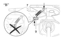
• Connect the spring 7 properly so that it does not jump off when the adjusting screw 9 is turned
