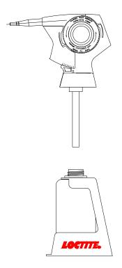
4. Screw pump to bottle until tight (approximately 13 in-lbs). If thread start is properly orientated the pump will face in the following position. If pump faces in the opposite direction unscrew pump, turn bottle 180 degrees and reassemble.
