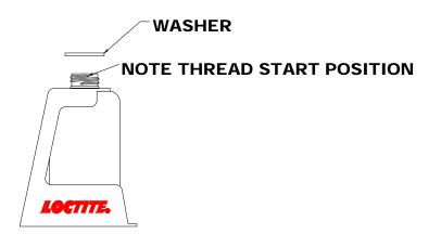
3. Insert pump tube into product bottle. Screw pump onto threaded neck of bottle.
