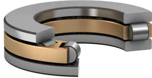
Single row cylindrical roller thrust bearings are designed to accommodate heavy axial loads and peak loads in one direction, but not radial loads. They provide a high degree of stiffness and require little axial space. They are mainly used in applications where thrust ball bearings do not have sufficient load carrying capacity. An important feature is the separable design, which facilitates mounting and enables the bearing components to be interchanged.
