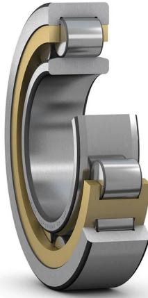
Single row cylindrical roller bearings are designed to accommodate high radial loads in combination with high speeds. Having two integral flanges on the outer ring and no flanges on the inner ring, NU design bearings can accommodate axial displacement in both directions. An important feature is the separable design, which facilitates mounting and enables the bearing components to be interchanged.
