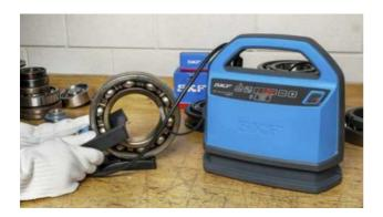
The TMBH 5 relies on an induction clamp that contains internal coils. A current in the coils generates a fluctuating magnetic field. This induces currents within the component, which are converted to heat. Because this heat is generated within the component – and not the clamp – the process is highly energy-efficient.
