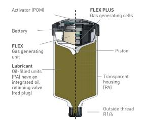
Dimensions FLEX FLEX 60: Ø 58 x 86.5 mm FLEX 125: Ø 58 x 117 mm
